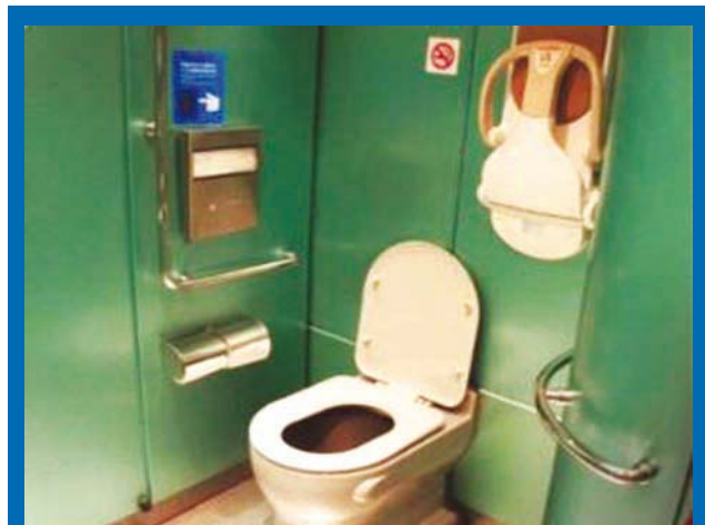
With an aim to provide clean and efficient toilets and to reduce the water consumption in toilets, IR is doing a trial of Bio-Vacuum Toilets. This has aircraft type vacuum toilet on the passenger interface and bio-digester tank is fitted beneath the toilet area on the coach.
